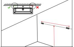
Mark the location of both mounting plates, ensuring that they are positioned inside the sidewalls of the unit. The recommended height for the unit including basin is 800-850mm.
